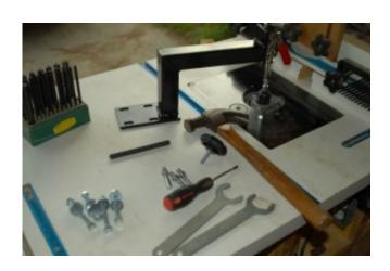
The next step was to mark where the four holes were to be drilled in the router table. I used a transfer punch to do this accurately. I drilled the holes carefully using a 5/16" bit. The directions called for using a 3/8" bit, but that seemed a bit big to me.
